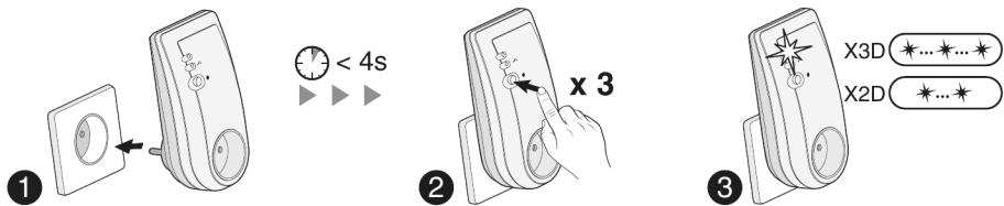
When switching on the installation (1), you have 4 seconds to press 3 times the receiver button (2). The LED flashes (3): 2 times for X2D, 3 times for X3D.
