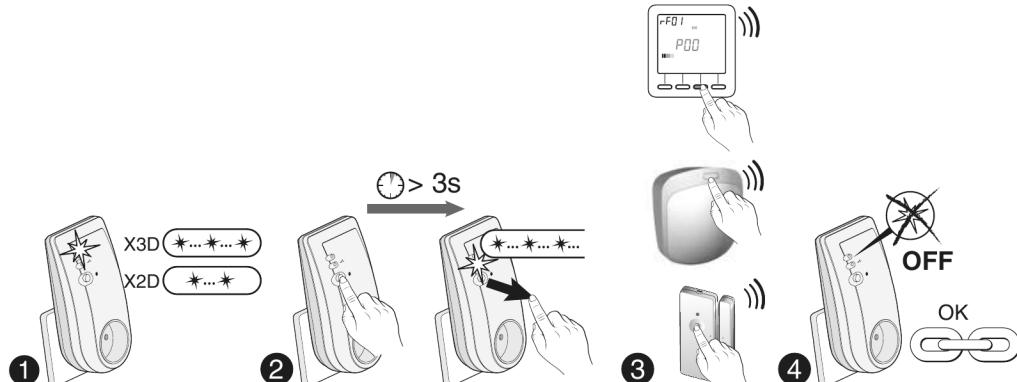
When switching on the installation (1) Wait until the LED flashes: 2 times (X2D) or 3 times (X3D).
